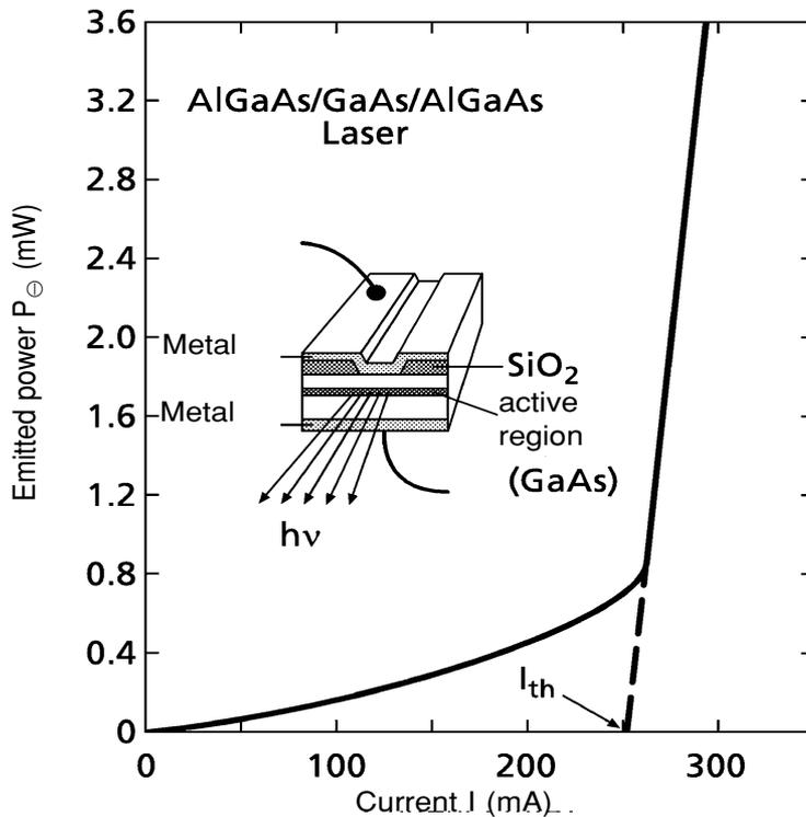
A further figure of merit of a semiconductor laser is the critical temperature  $T_0$ , which should be as high as possible because the threshold current  $I_{th}$  depends exponentially on the working temperature  $T$  as  $I_{th} \propto \exp(T/T_0)$ , so that the laser shows a slow increase of the threshold current with working temperature  $T$ . Typical values of  $T_0$  are close to 100°C for double heterostructure lasers.
