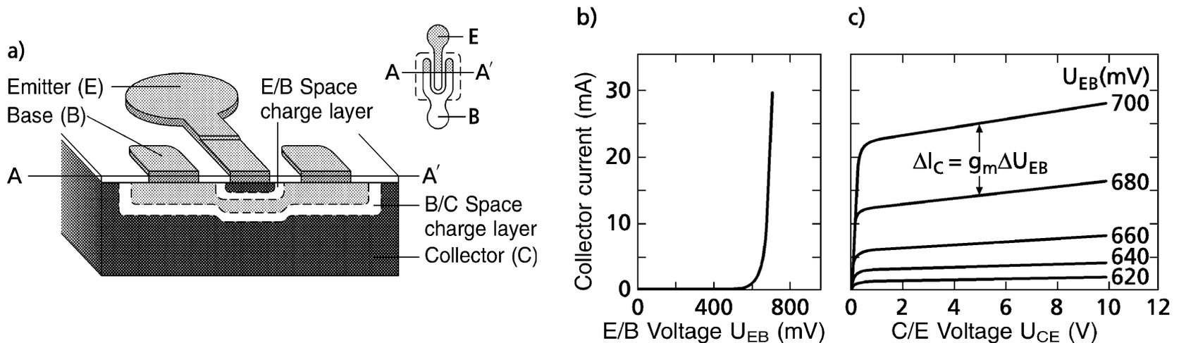
Significant voltage and power amplification can be achieved since the input circuit of the transistor contains the low-resistance emitter-base  $pn$  junction biased in the forward direction, while the output current  $I_C$  flows through the high resistance of the base-collector  $pn$  junction biased in reverse direction.
