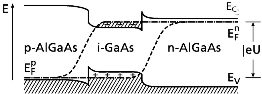
A lowly doped or intrinsic i-GaAs layer is inserted between two low  $p$ - and  $n$ -doped wide band gap AlGaAs regions.
