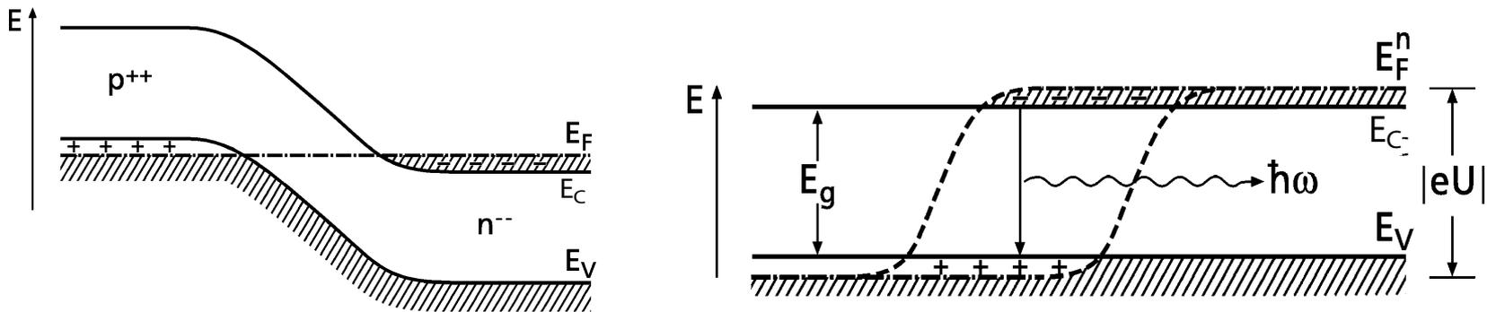
For laser operation, the quasi-Fermi levels in the  $n$ - and  $p$ -doped region must be separated from each other by more than the band gap energy  $E_g$ .
