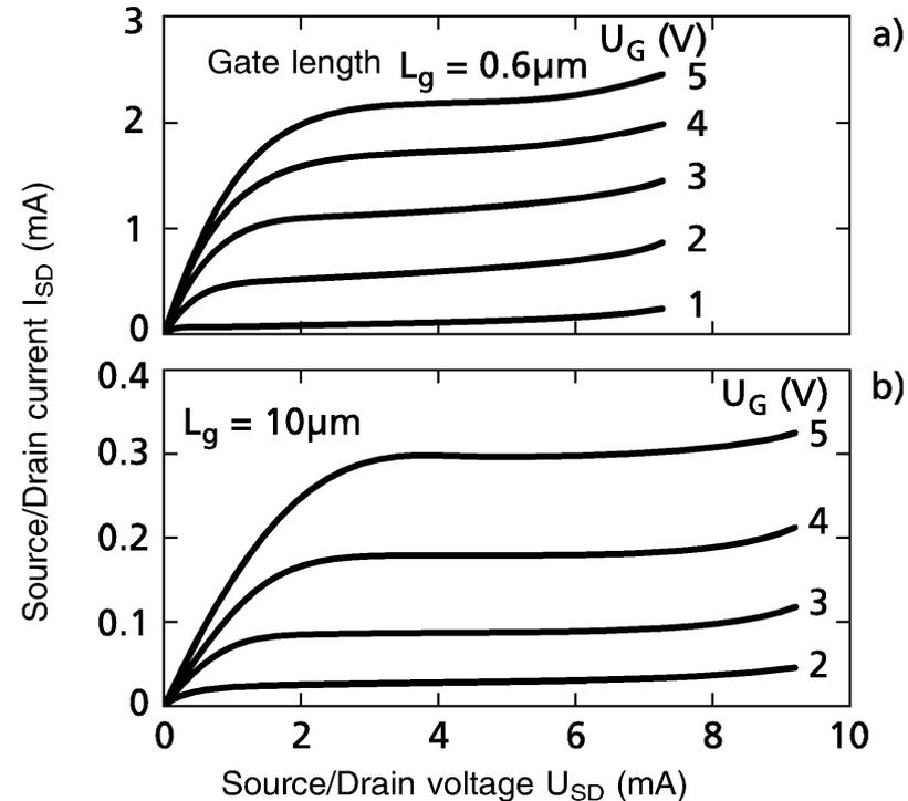
A bias voltage applied to the gate gives rise to a large electric field across the gate oxide layer that in turn causes a band bending in the underlying semiconductor. For a sufficiently positive gate voltage  $U_G$  the initial  $p$ -region (at  $U_G=0$ ) below the gate is inverted ( $E_i < E_F$ ) to become an  $n$ -accumulation layer. The two source and drain  $n^+$ -wells are thence connected by a conductive  $n$ -accumulation channel. The transistor has switched from "off" to "on".
