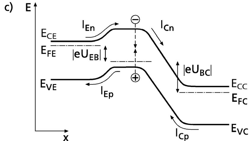
A scheme of an *npn*-transistor together with its external circuitry is shown: the first *n<sup>+</sup>p*-junction (emitter-base) is biased in the forward direction and the base-collector junction is biased in the reverse direction.
