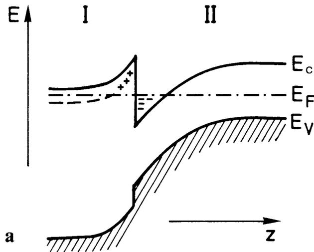
The high concentration of free electrons in this space-charge zone (semiconductor II) is compensated by a depletion space-charge zone in semiconductor I. In this way the high density of free electrons is spatially separated from the ionized impurities from which they originate.
