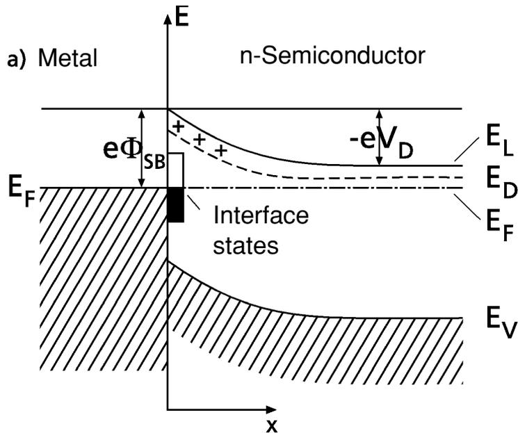
Conduction band states are negatively charged when occupied by electrons and neutral in the unoccupied state; valence band states, however are positive when empty and neutral in the occupied state. The band bending within the semiconductor is determined by a charge balance between negative charge  $Q_{is}$  in the interface states and the positive space charge  $Q_{SC}$  in the depletion layer.
